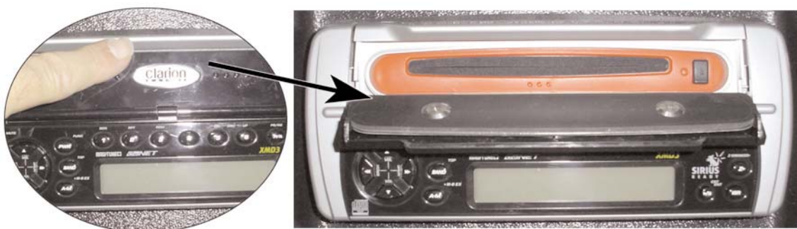
Figure 18. Opening the CD drive
